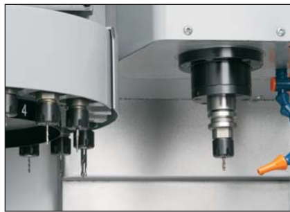
The OM-1A and OM-2A are equipped with a Haas-built, 30,000-rpm ISO 20-taper spindle and a 20-pocket automatic tool changer.
